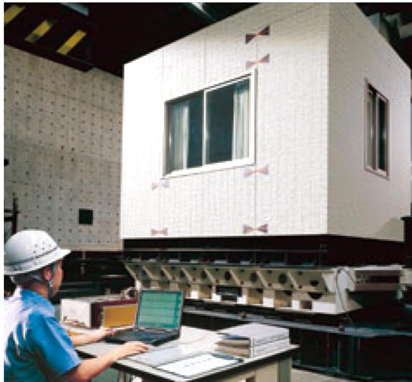
Life-size mockup at structural testing site that verifies seismic resistance levels
