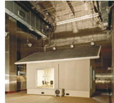
Test in an artificial climate room to verify insulation and comfort
